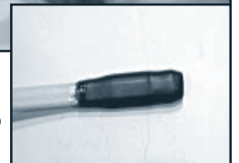
Step 21: Slide the over-cap over the end cap until fully seated.
