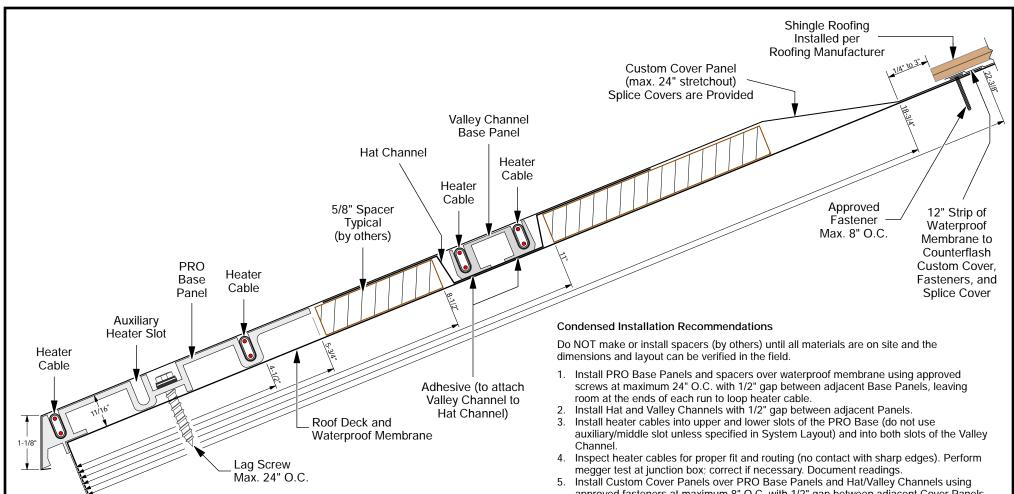
Install Custom Cover Panels over PRO Base Panels and Hat/Valley Channels using approved fasteners at maximum 8" O.C. with 1/2" gap between adjacent Cover Panels.
