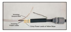
**9.** Slide and center 3" Heat Shrink Tube over the Insulated Step-Down Barrel Connectors. Apply heat evenly to shrink tubing around Heating Cable, Barrel Connectors, and Power Leads: (Waterproof Conduit for Power Supply by others not shown for clarity.)
