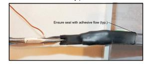
**10.** While the Heat Shrink Tubing is still hot, gently squeeze the tubing between the Power Leads with Needle Nose Pliers. The Heat Shrink Tubing must remain visibly sealed when the pliers are removed. If the Heat Shrink Tubing does not remain sealed, reheat the tubing and try again.
