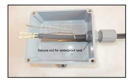
**8.** Feed incoming Power Leads through watertight conduit and connector (not shown for clarity). Strip Power Leads to expose 3/8" length of bare conductor. Insert bare conductors into open end of Insulated Barrel Connectors. Crimp across Yellow Stripe: (Junction Box not shown for clarity)
