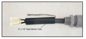
**7.** Insert assembly into bottom of NEMA 4 or 4X Electrical Junction Box (provided by others) and tighten nut and all fittings to create a watertight seal. Junction Box should be protected from weather, if possible:
