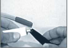
**Step 17:** Put a small amount of RTV into the opening of the larger over-cap.
