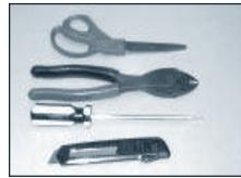
**Tools Required for Installation** Scissors, crimper/cutter, flat-blade screwdriver, and utility knife
