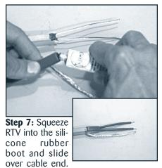
Verify bus wires do not contact ground wire.
