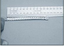
**Step 2:** Cut overjacket back a distance of 5" (120 mm).
