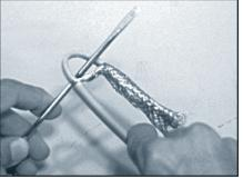
**Step 3:** Separate braid strands at overjacket and pull cable back through opening in braid.
