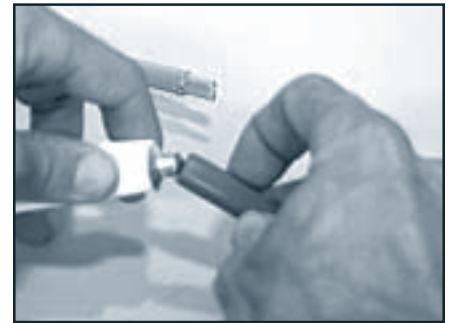
Step 18: Fill the smaller end cap with RTV.
